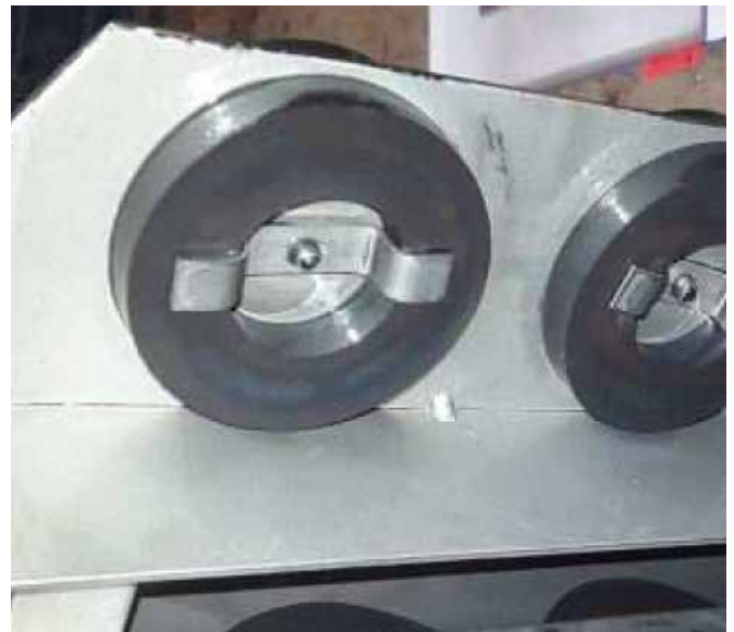
Magnetic insert after cleaning
