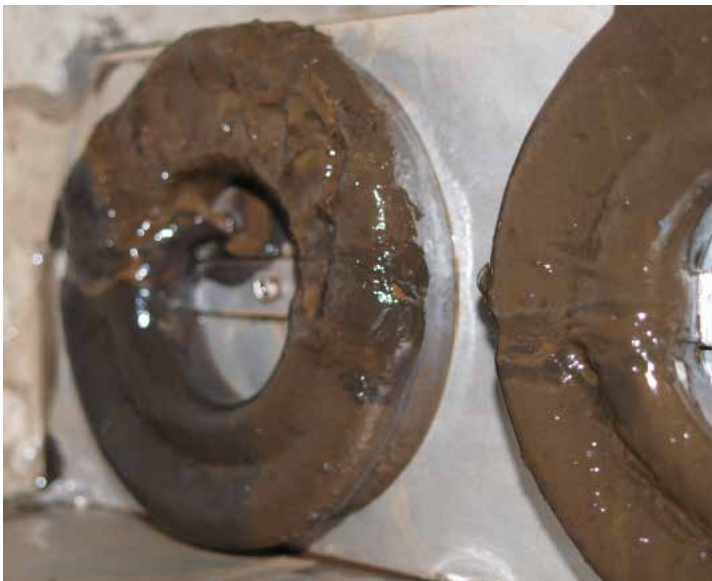
Magnetic insert before cleaning
