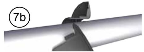
The rosettes can be opened and closed along their circumference (7b). This allows them to be fitted or exchanged even where the pipes have already been connected.
