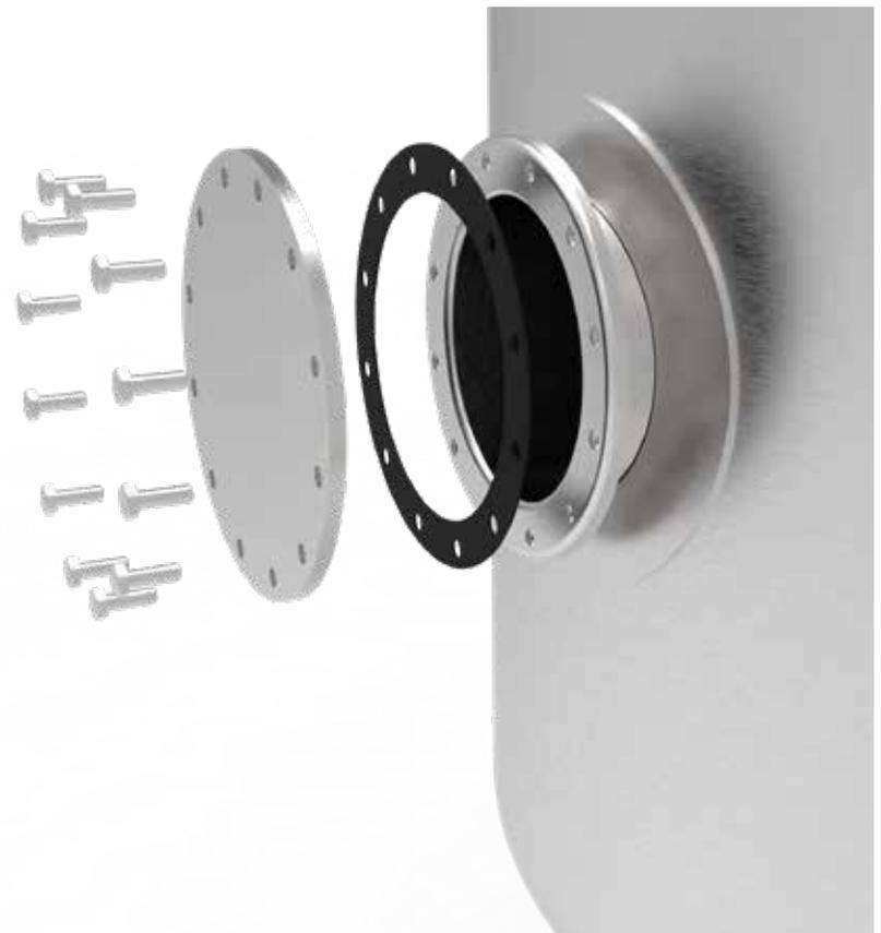
**Before starting-up the pressure vessels it is absolutely necessary to re-tighten the bolts!**
